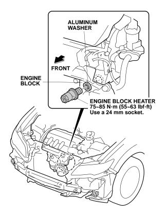
18. Plug the heater harness connector into the engine block heater.
