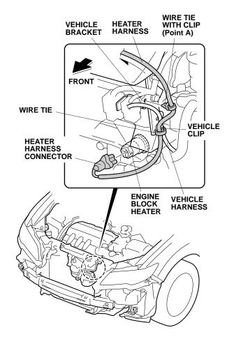
19. Route the heater harness in the direction shown, and secure the wire tie with clip (point A) to the vehicle bracket. Secure the heater harness to the vehicle harness with one wire tie.
