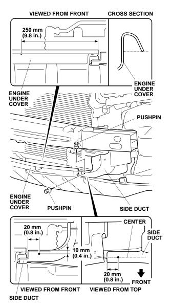
13. While wearing eye protection, drill the three pierced marks on the side duct and engine under cover with a 3 mm drill bit, then enlarge the three holes with a 7 mm drill bit. Remove any burrs. Wrap tape around each drill bit 7 mm away from the tip or use a drill stop.
