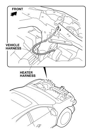
22. Route the heater harness under the left headlight, and secure it to the side duct with one black wire tie (point C).
