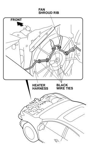
29. With the help of an assistant, route the heater harness through the front bumper opening, and reinstall the front bumper.
