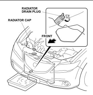
4. After the coolant drains, reinstall the radiator cap to prevent dirt and contamination from entering the radiator.
